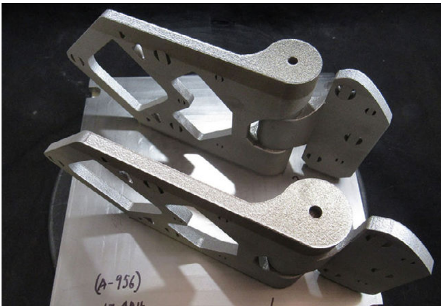
Figure 4: Optimized geometry of the additively manufactured hinge, which reduced hinge weight by 38% from the original hinge assembly
