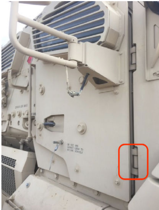
Figure 1: A picture of the cab door hinge on an Army MRAP vehicle.
